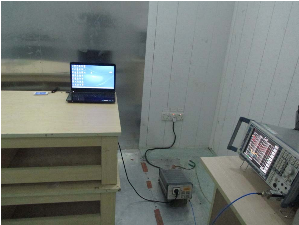
FCC RADIATED EMISSION TEST SETUP
