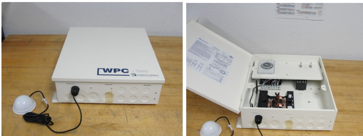
FIGURE 27: WPC-2 Repeater and Relay Controller
