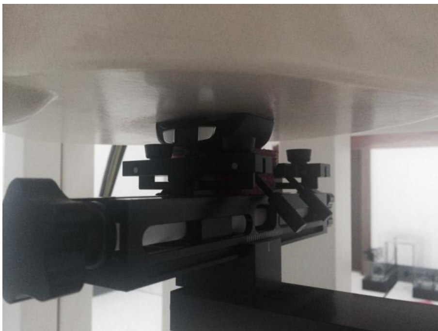
Wrist-Worn with gap 0mm (Flat Phantom)
