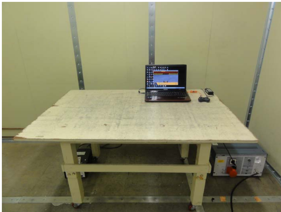
Photograph 4 : Setup for AC Conducted Emissions
