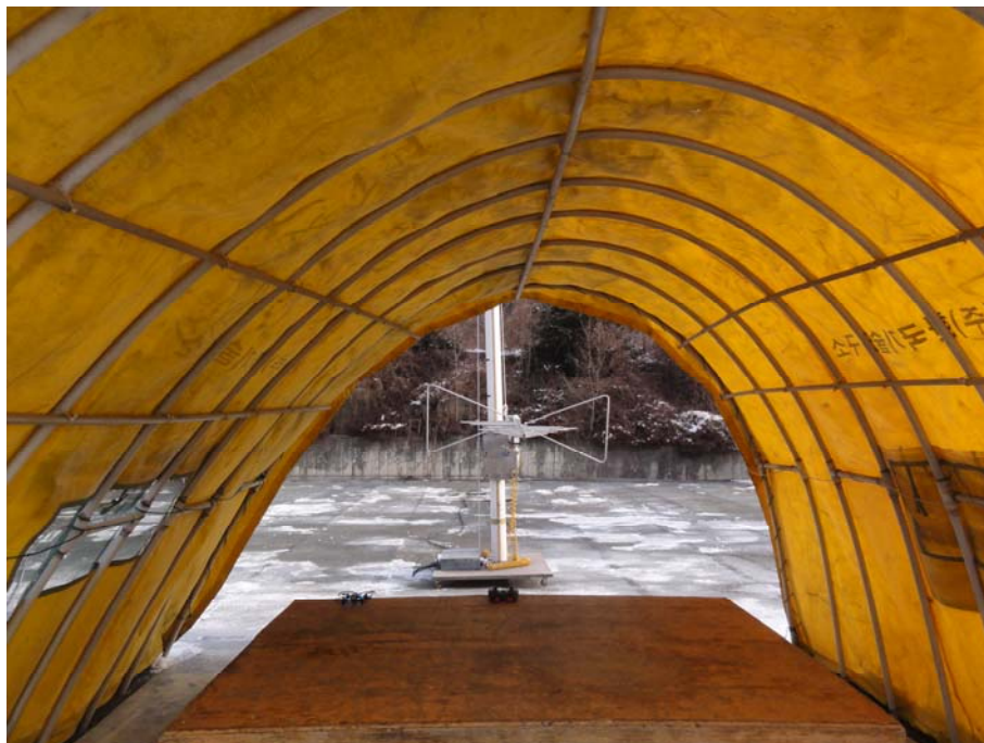
Photograph 2 : Setup for radiated Emissions (above 1 GHz)
