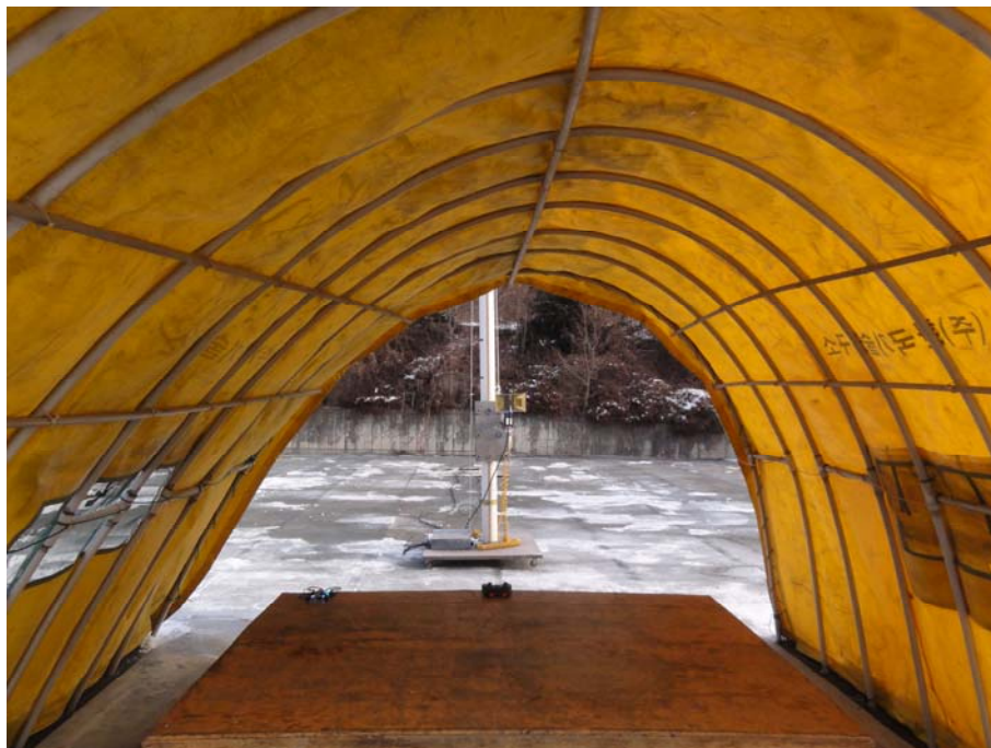
Photograph 3 : Setup for radiated Emissions (above 1 GHz)
