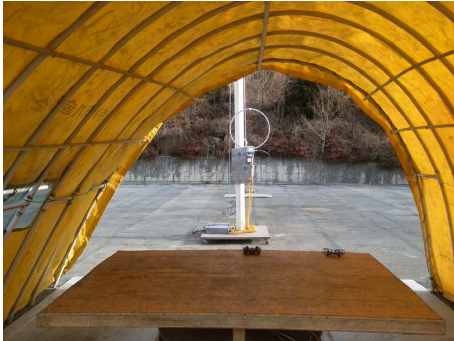
Photograph 1 : Setup for radiated Emissions (above 30 MHz)
