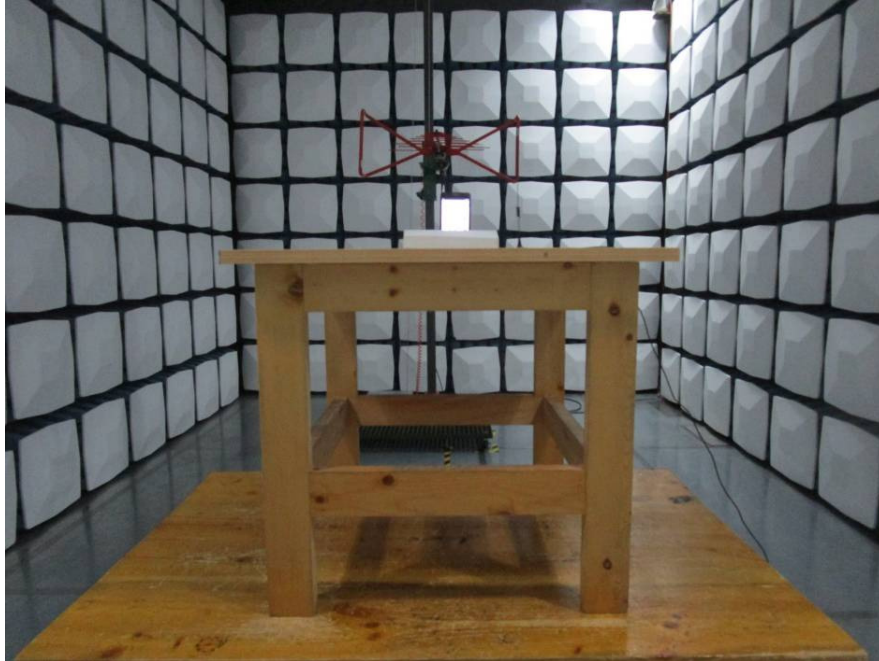
Radiated Emission View---Below 1GHz
