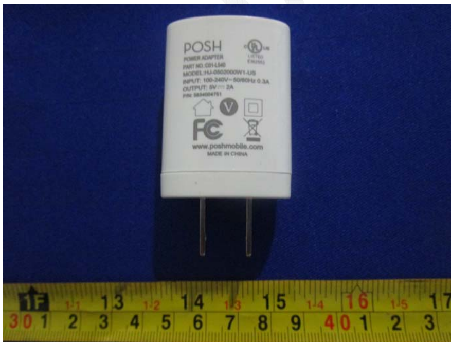
EUT –Adapter Top View
