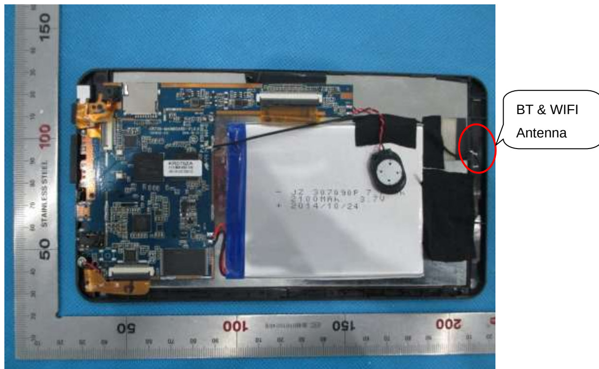
INTERNAL VIEW OF EUT-1
