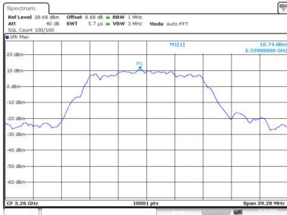
PSD NVNT 802.11a 5260MHz Ant1
