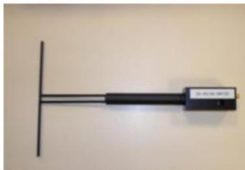
Figure 1 – Satimo COMOSAR Validation Dipole
