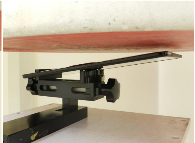
Bottom - Slant of Edge2, Test Separation 1.3 cm
