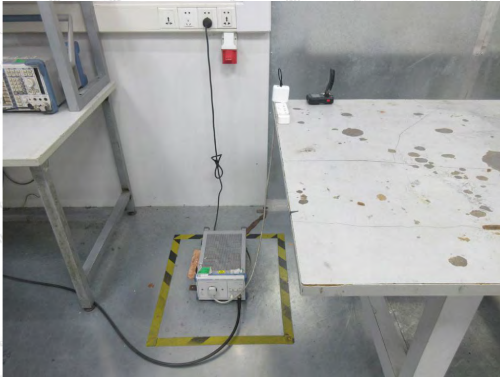
Photo of Power Line Conducted Emission Test
