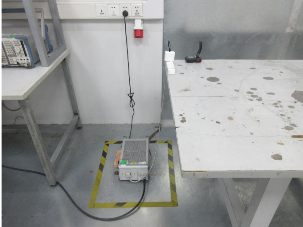
Photo of Power Line Conducted Emission Test
