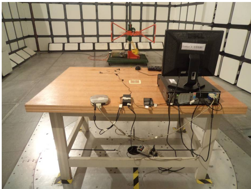
Radiated Emissions – Rear View (Below 1 GHz)
