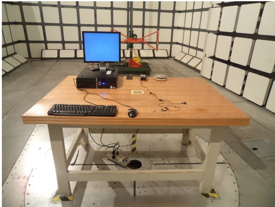
Radiated Emissions – Front View (Below 1 GHz)
