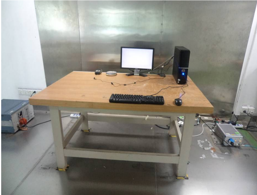
Conducted Emissions - Front View
