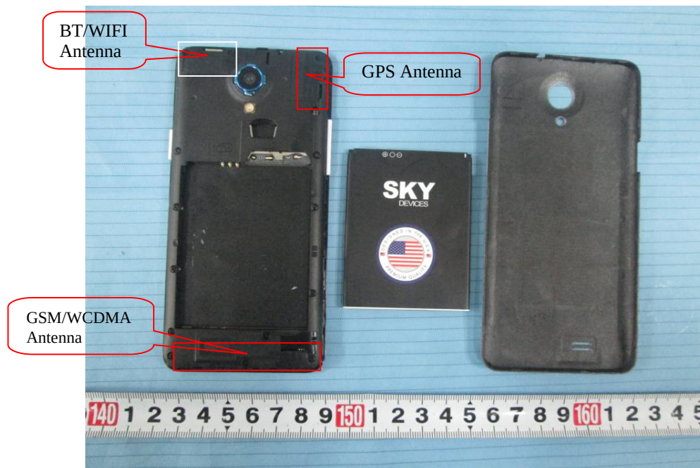
EUT –Cover off View 1
