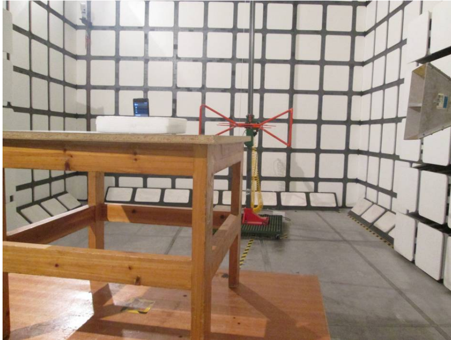
Radiated Emissions Test View (Below 1 GHz)
