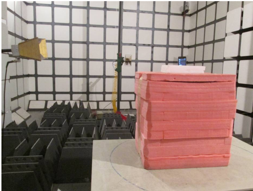
Radiated Emissions Test View (Above 1 GHz)
