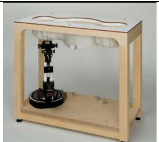
Fig. 8.7 Photo of SAM Twin Phantom
