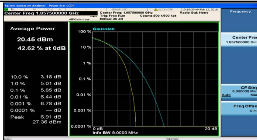
(Channel Bandwidth:15 MHz)_LCH_16QAM_75RB#0
