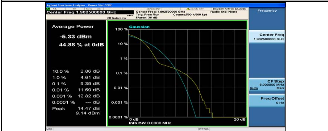
(Channel Bandwidth:15 MHz)_HCH_16QAM_1RB#37
