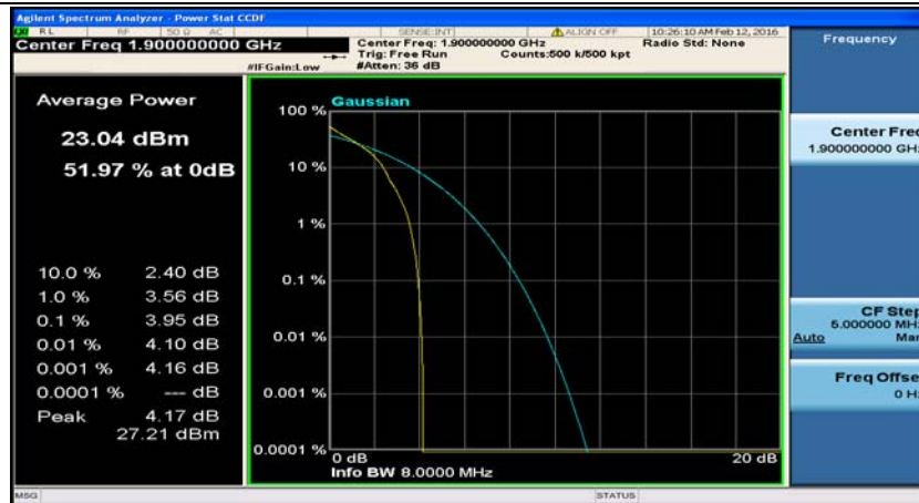
(Channel Bandwidth:20 MHz)_HCH_QPSK_1RB#99
