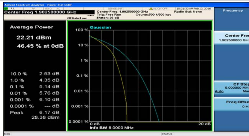
(Channel Bandwidth:15 MHz)_HCH_QPSK_37RB#38
