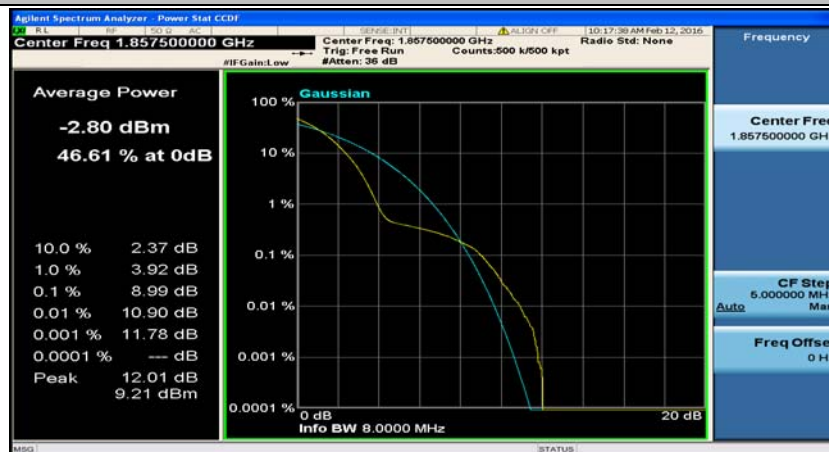
(Channel Bandwidth:15 MHz)_LCH_QPSK_37RB#0
