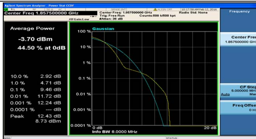
(Channel Bandwidth:15 MHz)_LCH_16QAM_37RB#0
