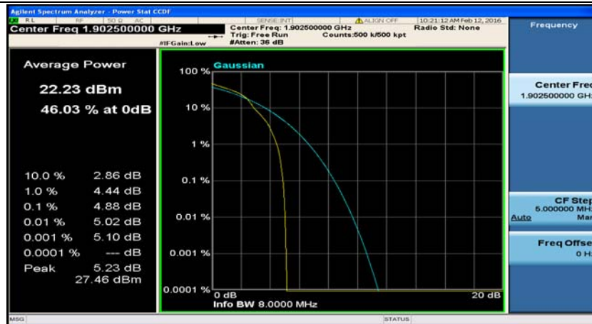
(Channel Bandwidth:15 MHz)_HCH_16QAM_1RB#74
