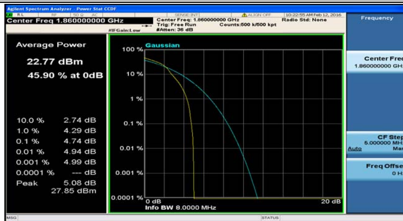
(Channel Bandwidth:20 MHz)_LCH_16QAM_1RB#99
