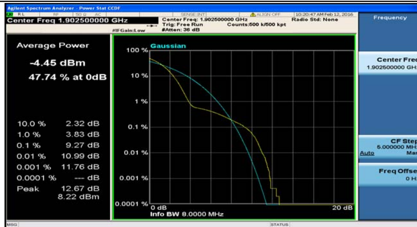
(Channel Bandwidth:15 MHz)_HCH_QPSK_1RB#37
