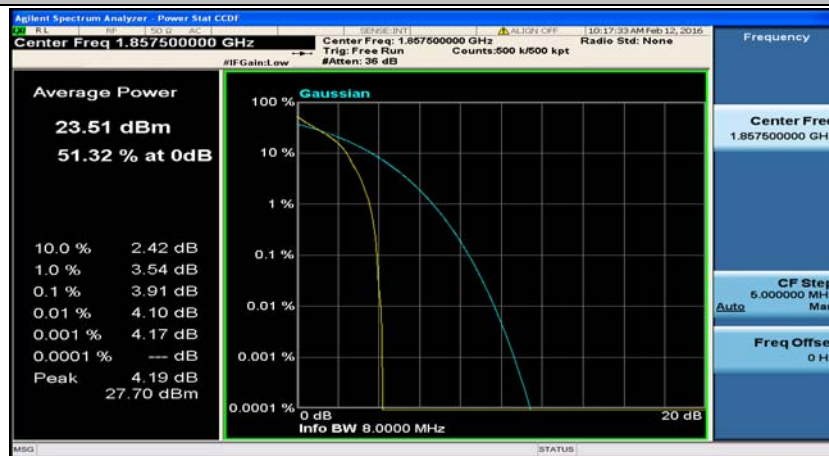
(Channel Bandwidth:15 MHz)_LCH_QPSK_1RB#74
