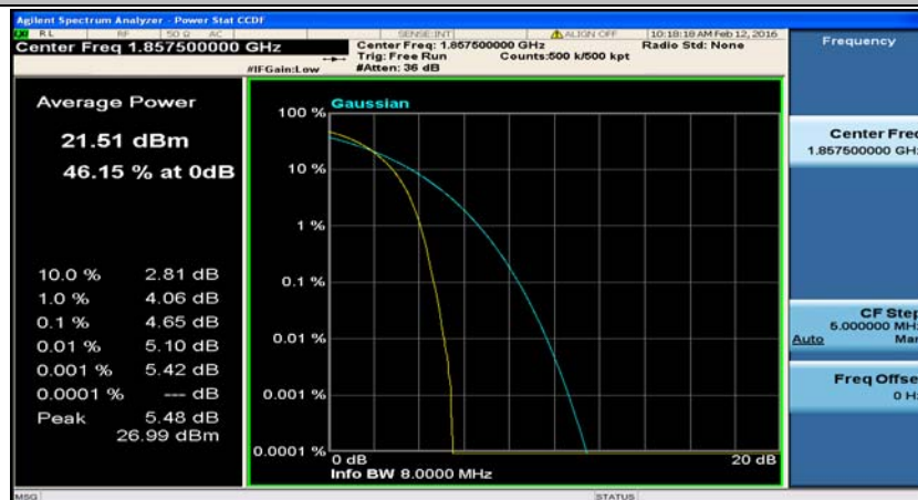
(Channel Bandwidth:15 MHz)_LCH_QPSK_75RB#0
