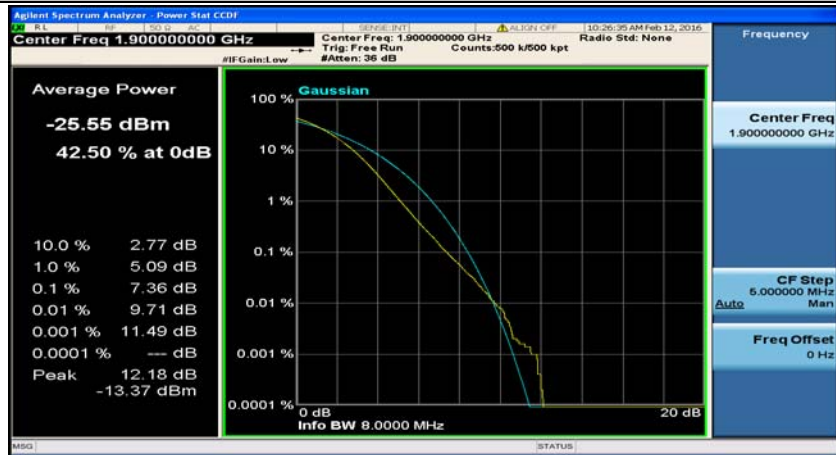
(Channel Bandwidth:20 MHz)_HCH_16QAM_50RB#0
