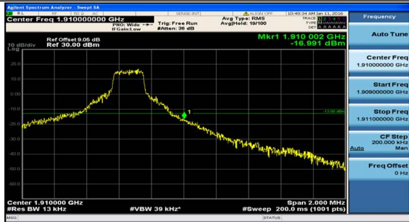
(Channel Bandwidth: 5 MHz)_HCH_16QAM_12RB#0
