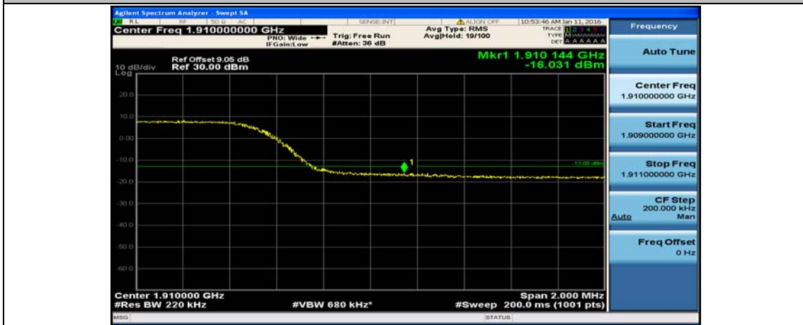
Channel Bandwidth: 10 MHz_HCH_QPSK_50RB#0
