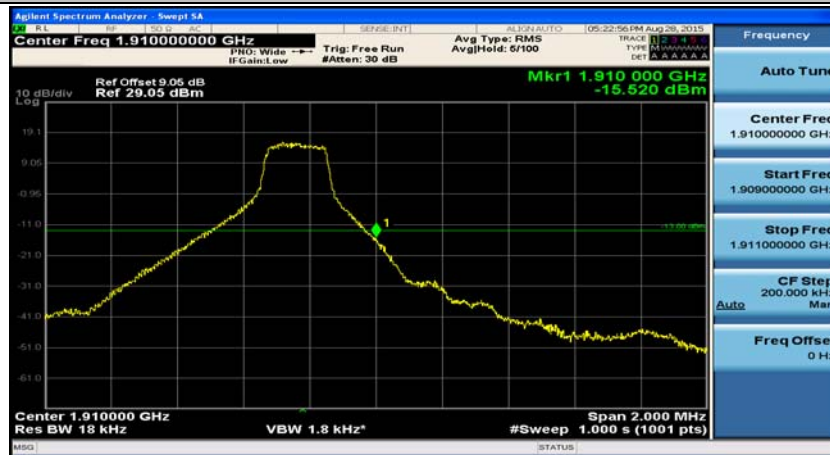
(Channel Bandwidth: 3 MHz)_HCH_QPSK_8RB#0
