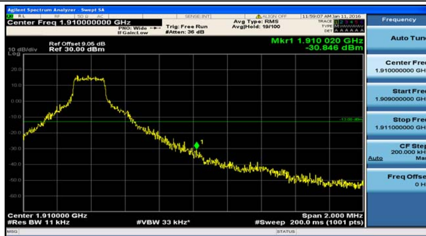
(Channel Bandwidth: 1.4 MHz)_HCH_16QAM_1RB#5
