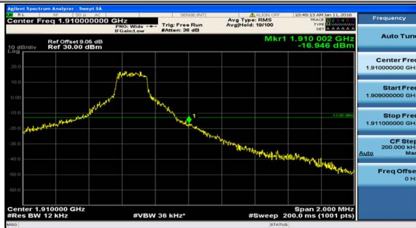
(Channel Bandwidth: 5 MHz)_HCH_QPSK_12RB#0
