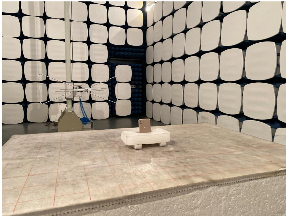
Radiated Spurious Emission Below 1GHz
