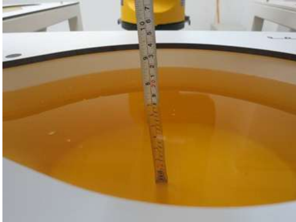
Fig. 9.1 Photo of Liquid Height for Head SAR
