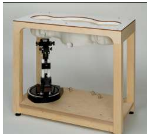
Fig. 8.7 Photo of SAM Twin Phantom
