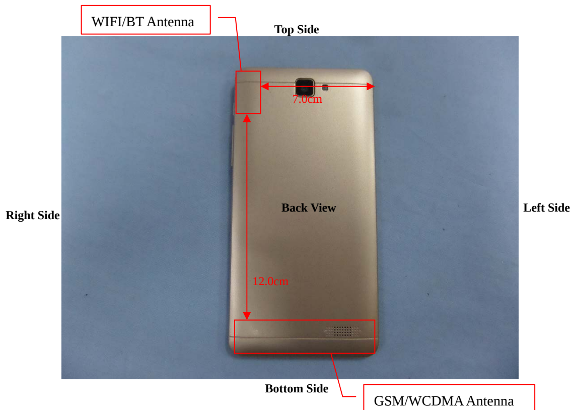
Block Diagram for EUT Antenna Position
