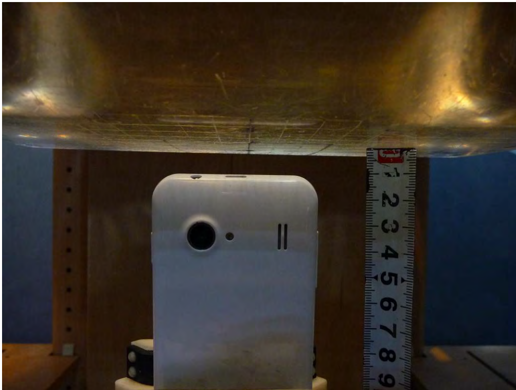
Body-worn Top Setup Photo (10mm)
