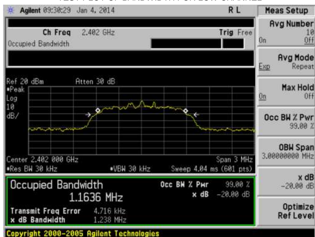
TEST PLOT OF BANDWIDTH FOR LOW CHANNEL
