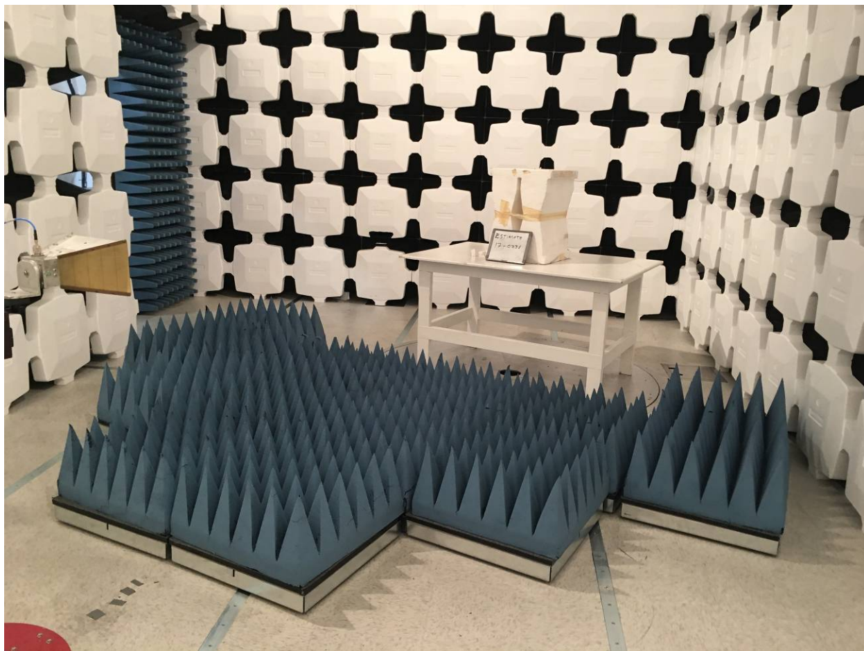
Figure 2. Intentional Radiated Emissions Test Setup, Above 1GHz (Fundamental and Harmonics)
