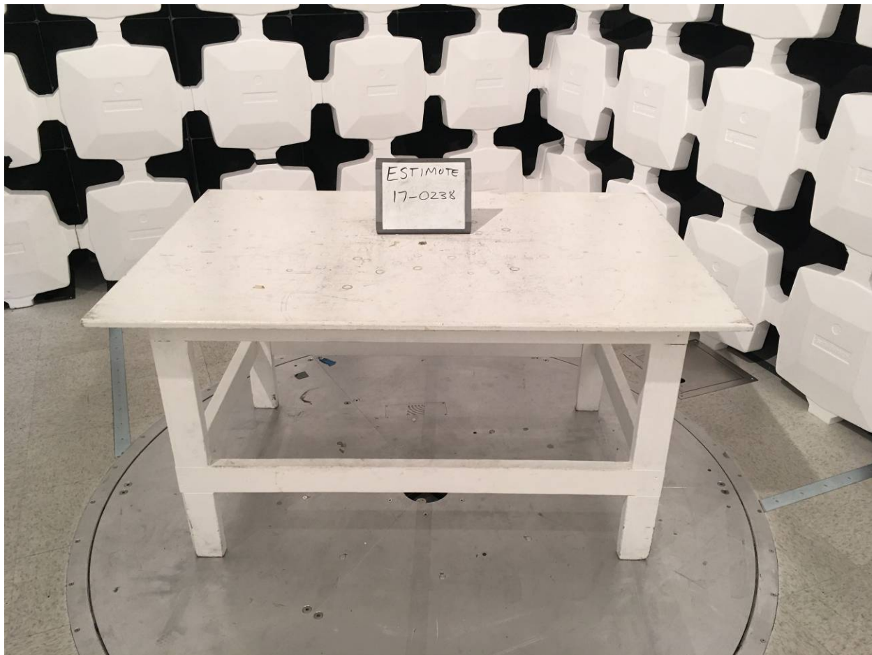
Figure 6. Unintentional Radiated Emissions Test Configuration Setup
