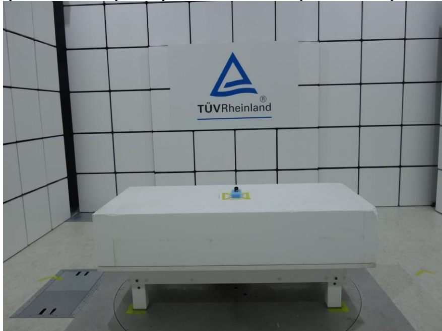
Photograph 2: Test Setup for Spurious Emissions (Front View 2)
