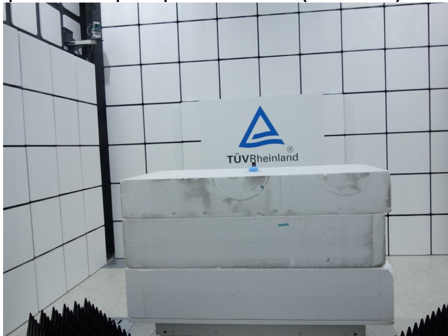
Photograph 2: Test Setup for Spurious Emissions (Front View 2)
