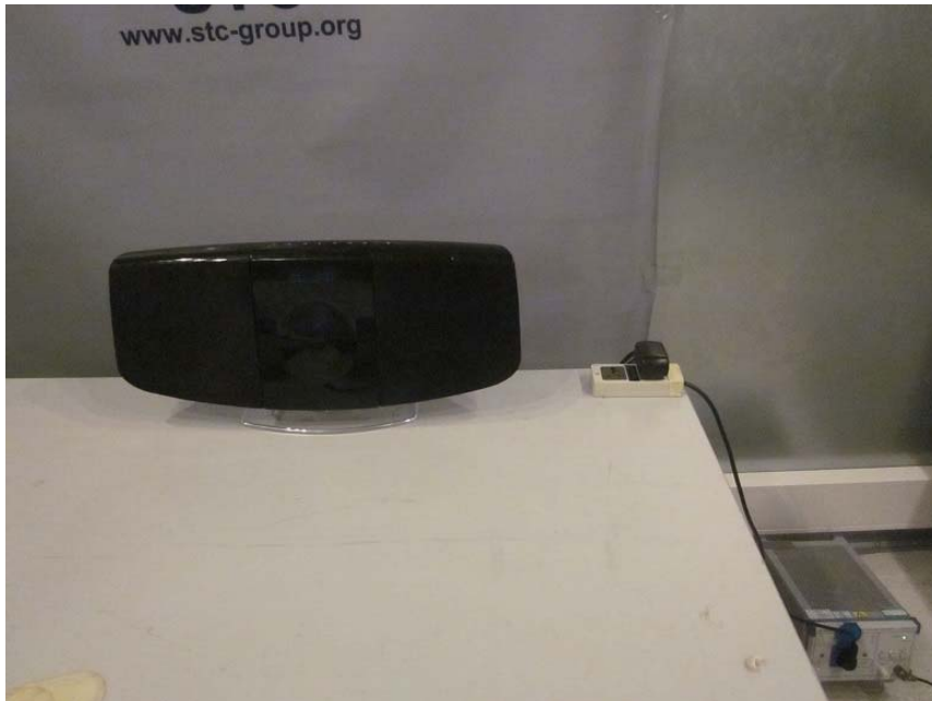
Measurement of Conducted Emission Test Set Up
