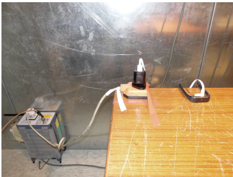
Set-up for AC mains Conducted Emission (Charging mode)
