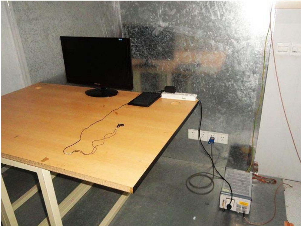
Conducted Emission Test Setup:
