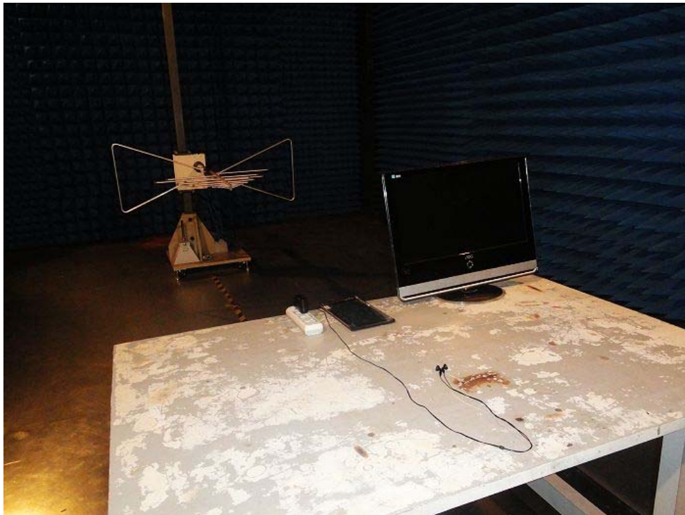
Radiated Emission Test Setup:
