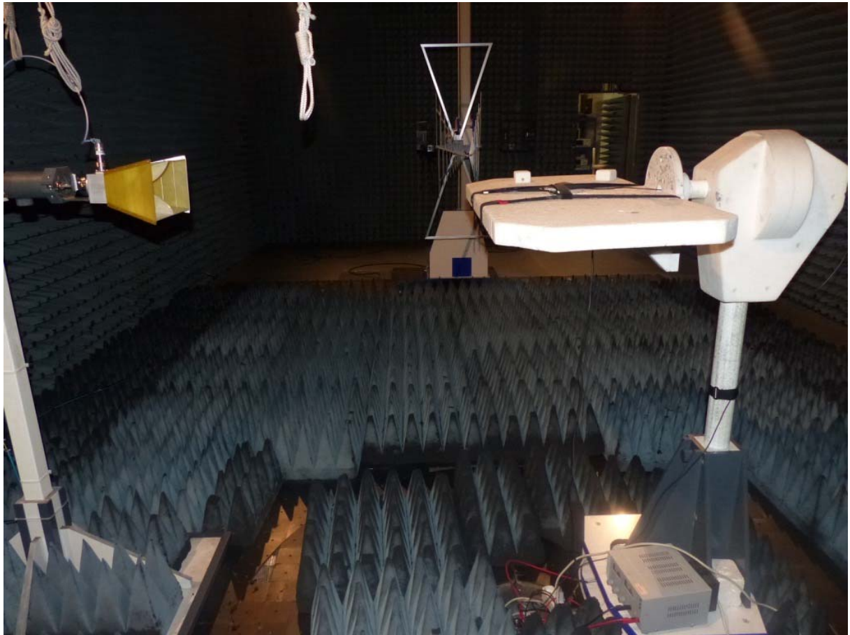
Photo 3: Test setup for radiated measurements (Enclosure, fully-anechoic chamber, 1-15 GHz intentional radiator §15, ANSI C63.10)
