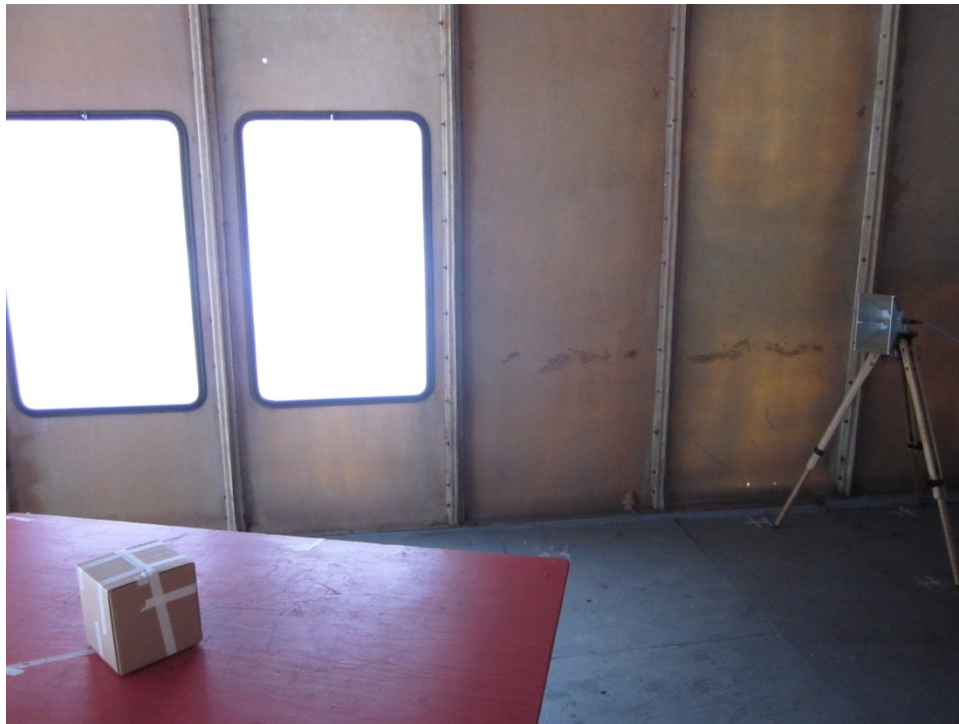
Oats Setup, 1 GHz to 18 GHz, Horizontal Polarization, Model: TB-200
