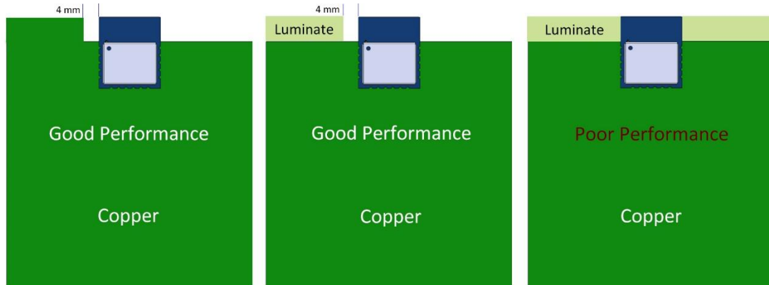
Figure 10: Antenna Performance Proximity with Copper (Left), Laminate (Middle) and Laminate Under Antenna (Right)
