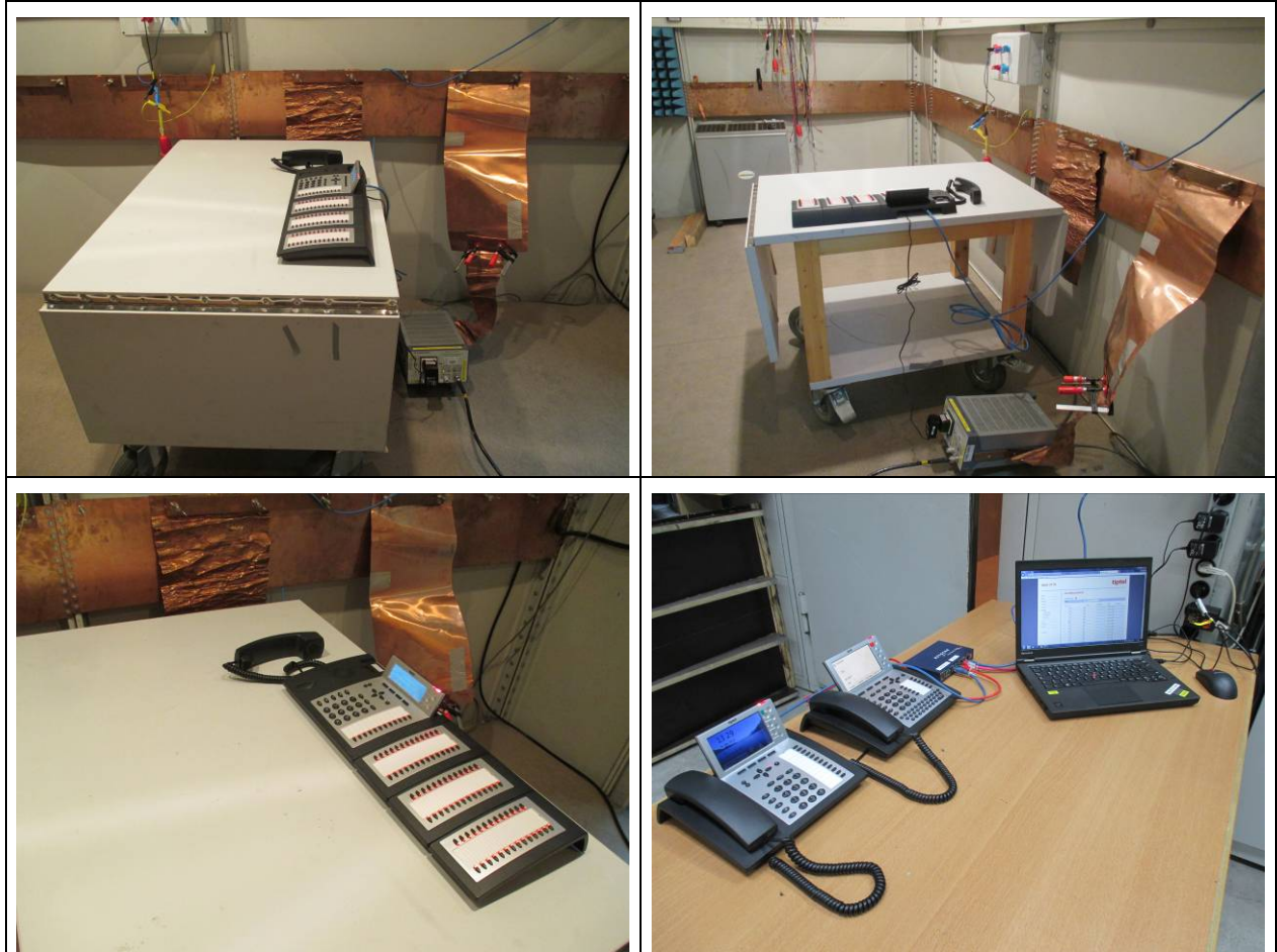
Figure 7-6: Test Setup Conducted Emissions (150 kHz – 30 MHz)
