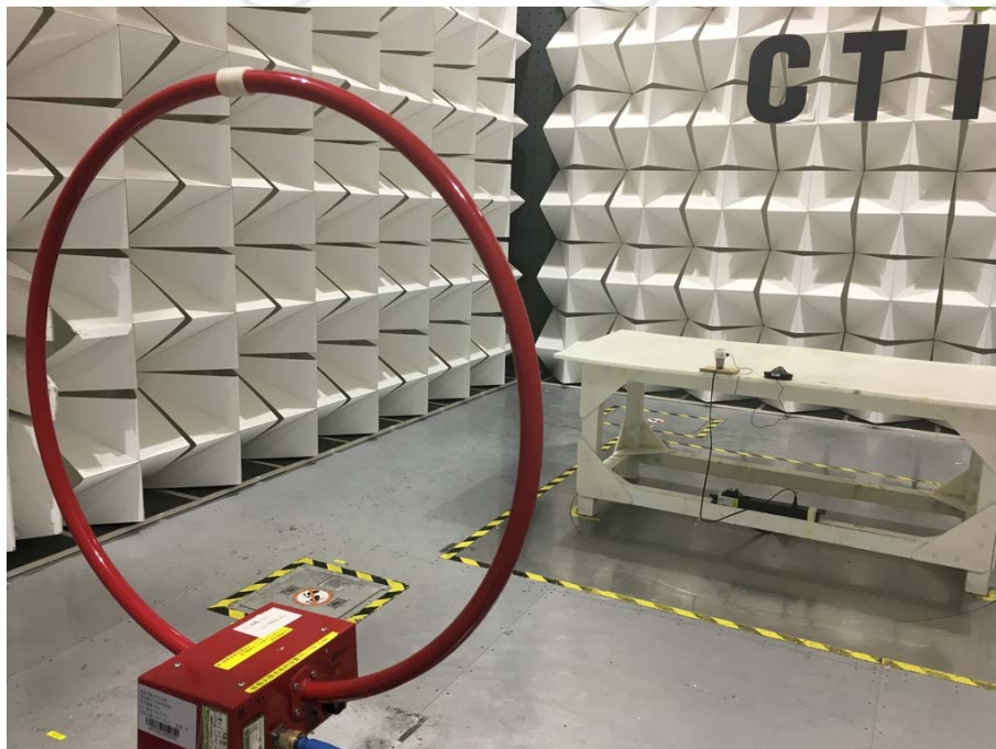
Radiated spurious emission Test Setup-1(Below 30MHz)
