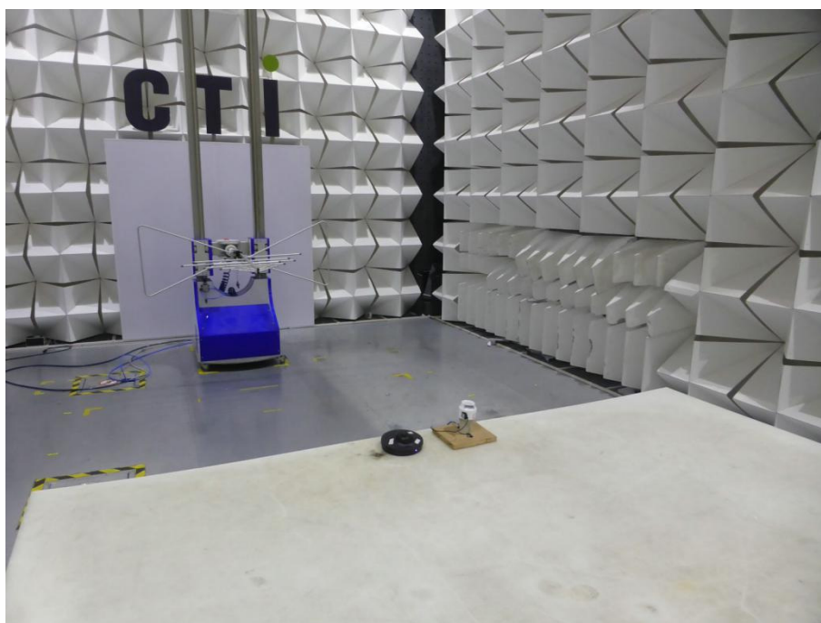
Radiated spurious emission Test Setup-2(30MHz-1GHz)
