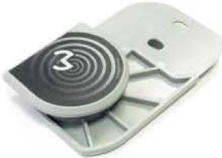
Figure 7: Door RFID Antenna – top side
