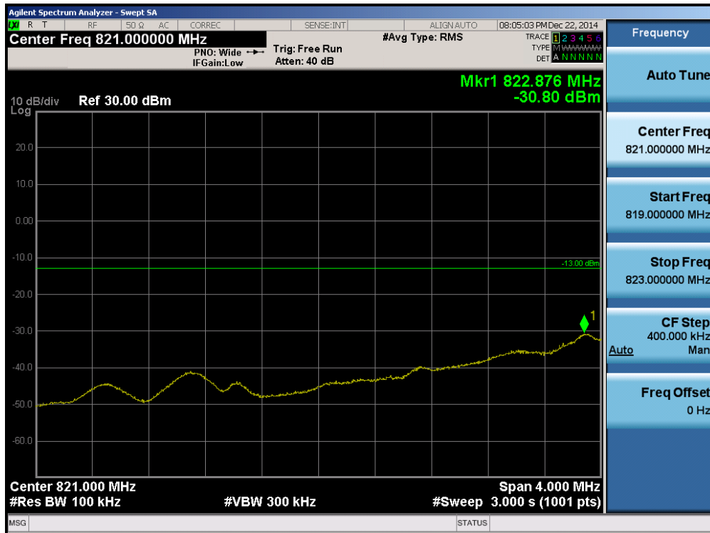
Plot 7-16. 4MHz Span Plot (Cellular CDMA Mode – Ch. 1013)
