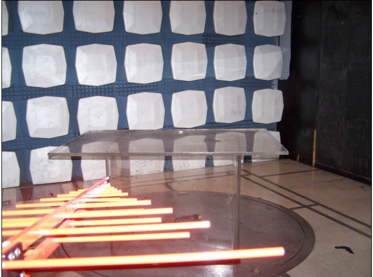
Photograph 2. Radiated Emissions, Test Setup
