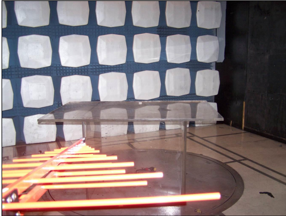
Photograph 3. Radiated Spurious Emissions, 30MHz-1GHz, Test Setup
