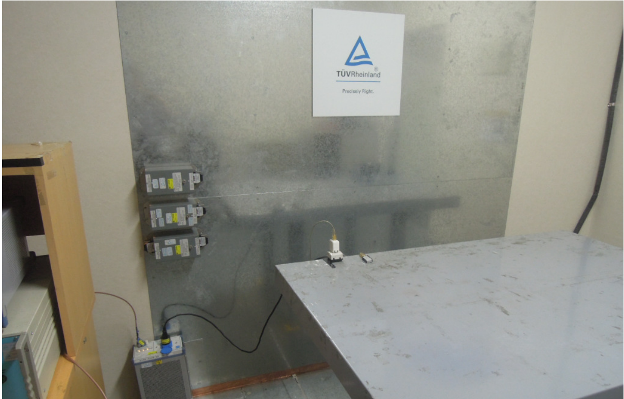
Photograph 8: Set-up for Mains Conducted testing Front
