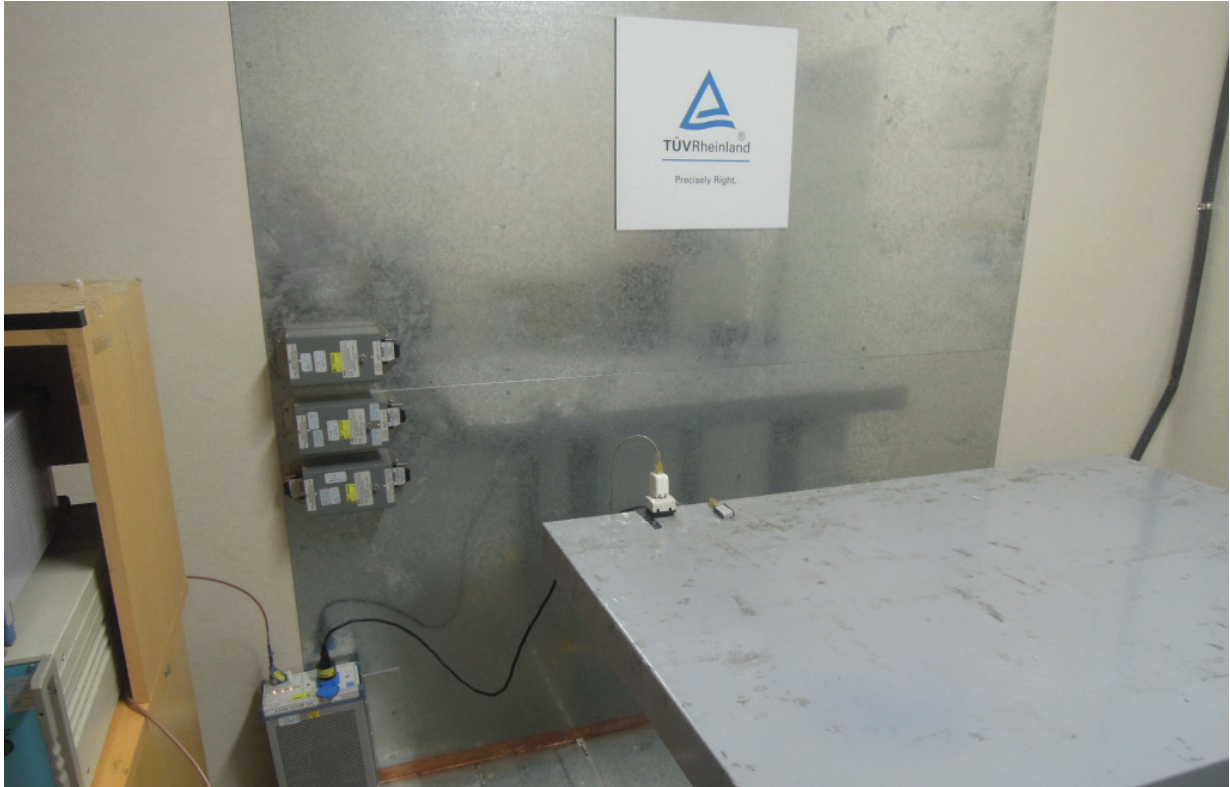
Photograph 8: Set-up for Mains Conducted testing Front
