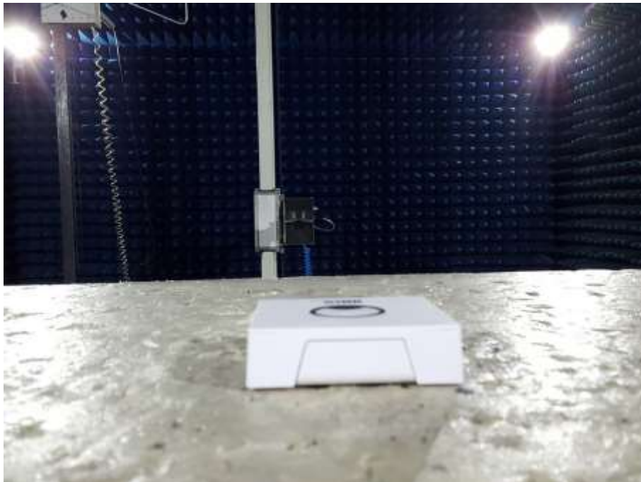
Photograph 3: Set-up for Radiated Spurious Emission (1GHz ~ 18GHz)
