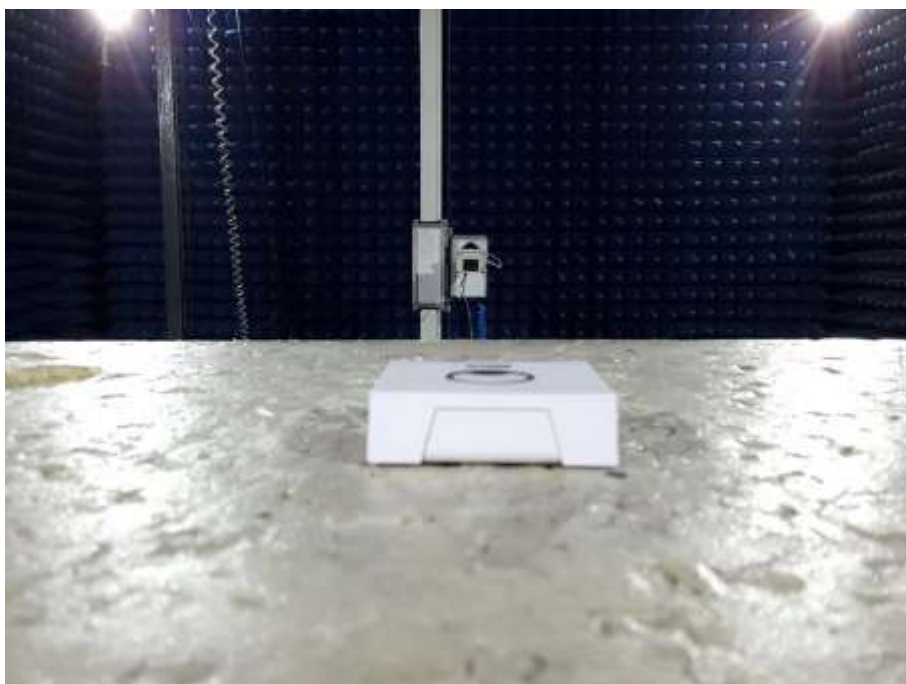
Photograph 4: Set-up for Radiated Spurious Emission above 18GHz
