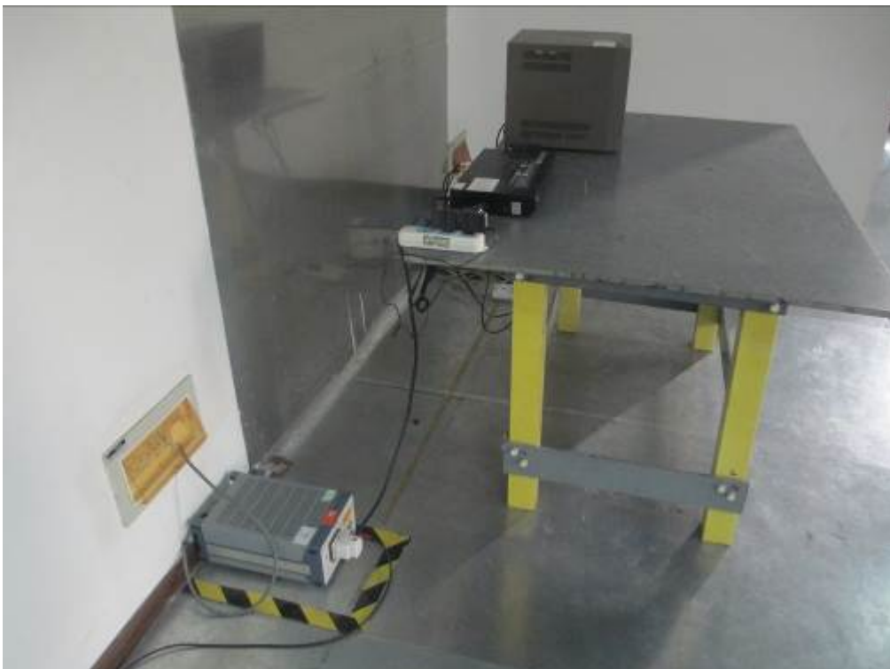
Conducted Emissions Test Setup Side View
