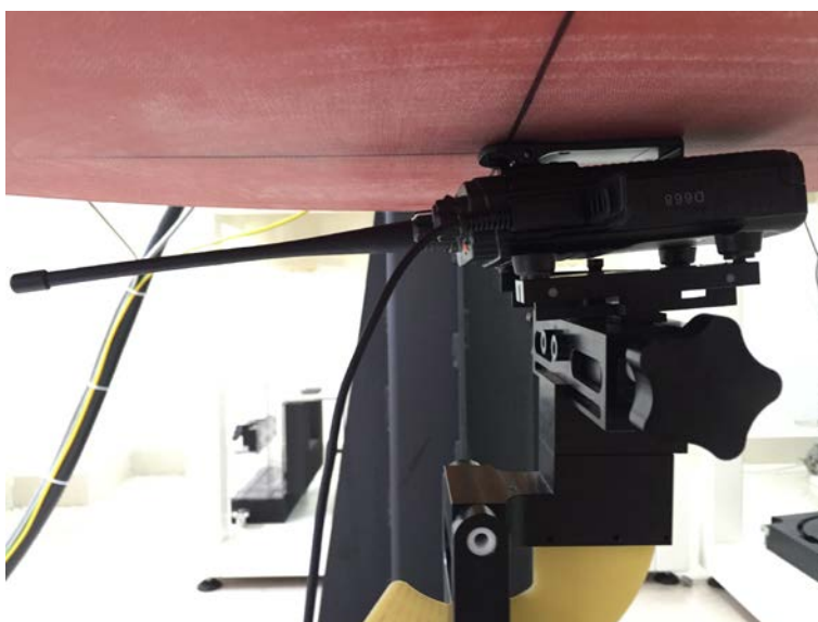
Body-worn, the front of the EUT towards ground with A1, B1, BC1 and AC1
