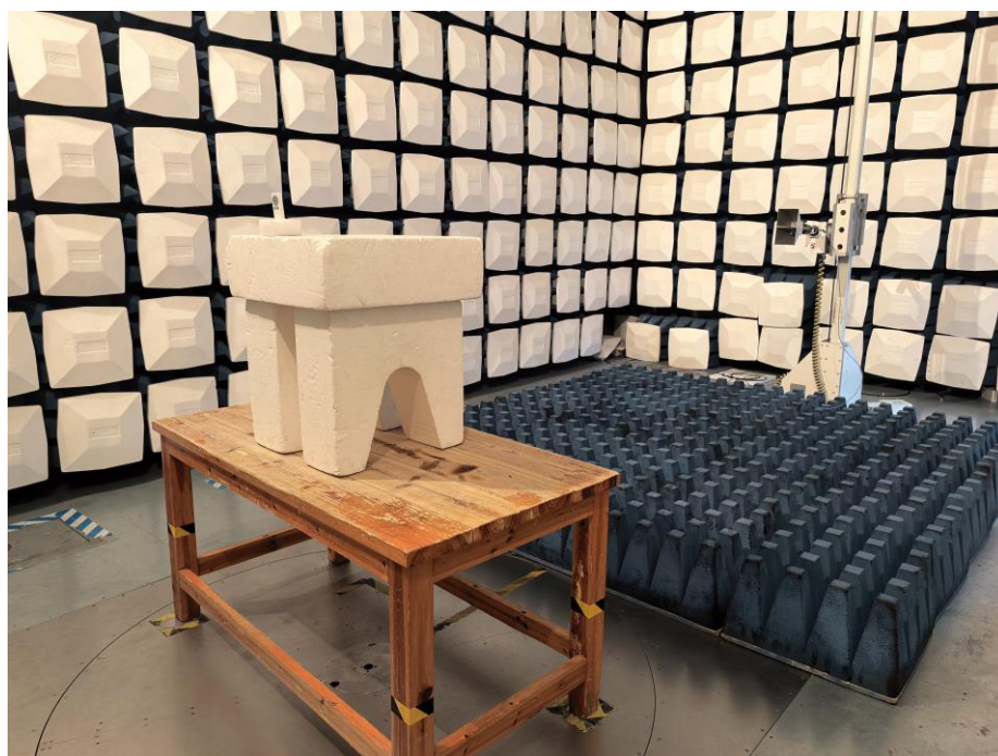
Test Setup For Radiated Emission (Above 1GHz)
