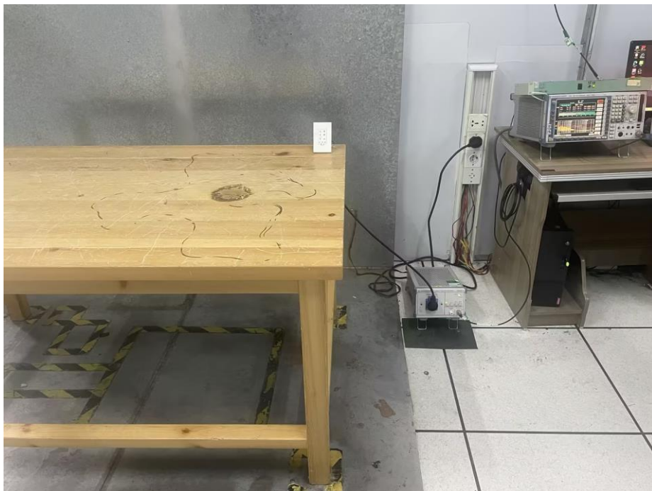
Test Setup For Conducted Emission
