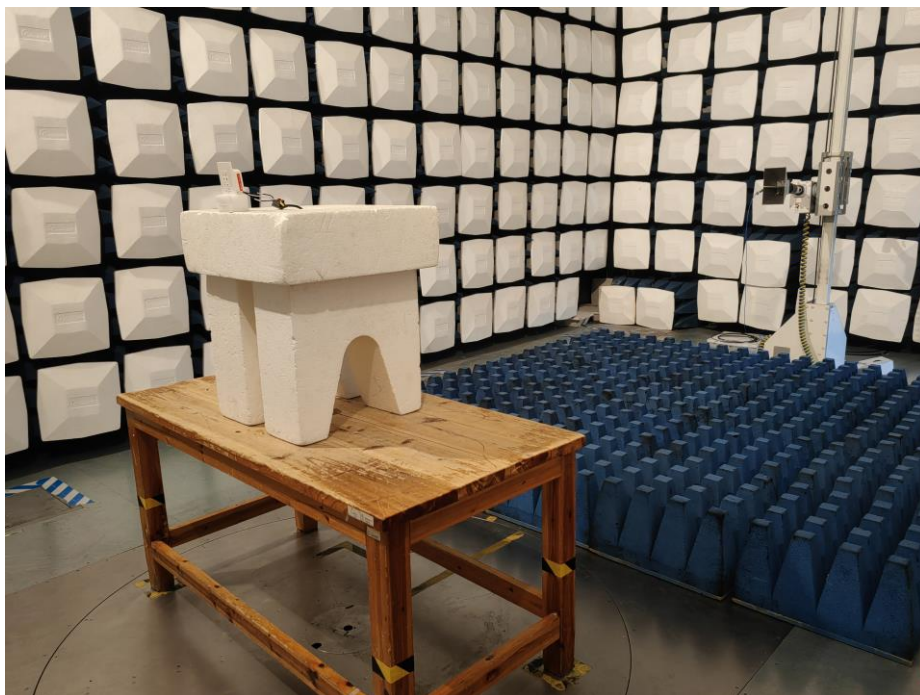
Test Setup For Radiated Emission (Above 1GHz)
