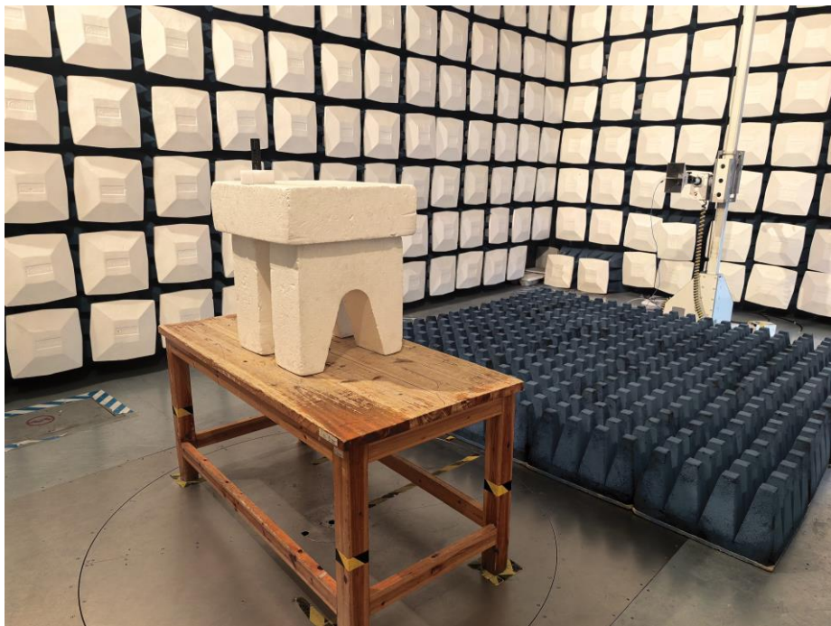
Test Setup For Radiated Emission (Above 1GHz)
