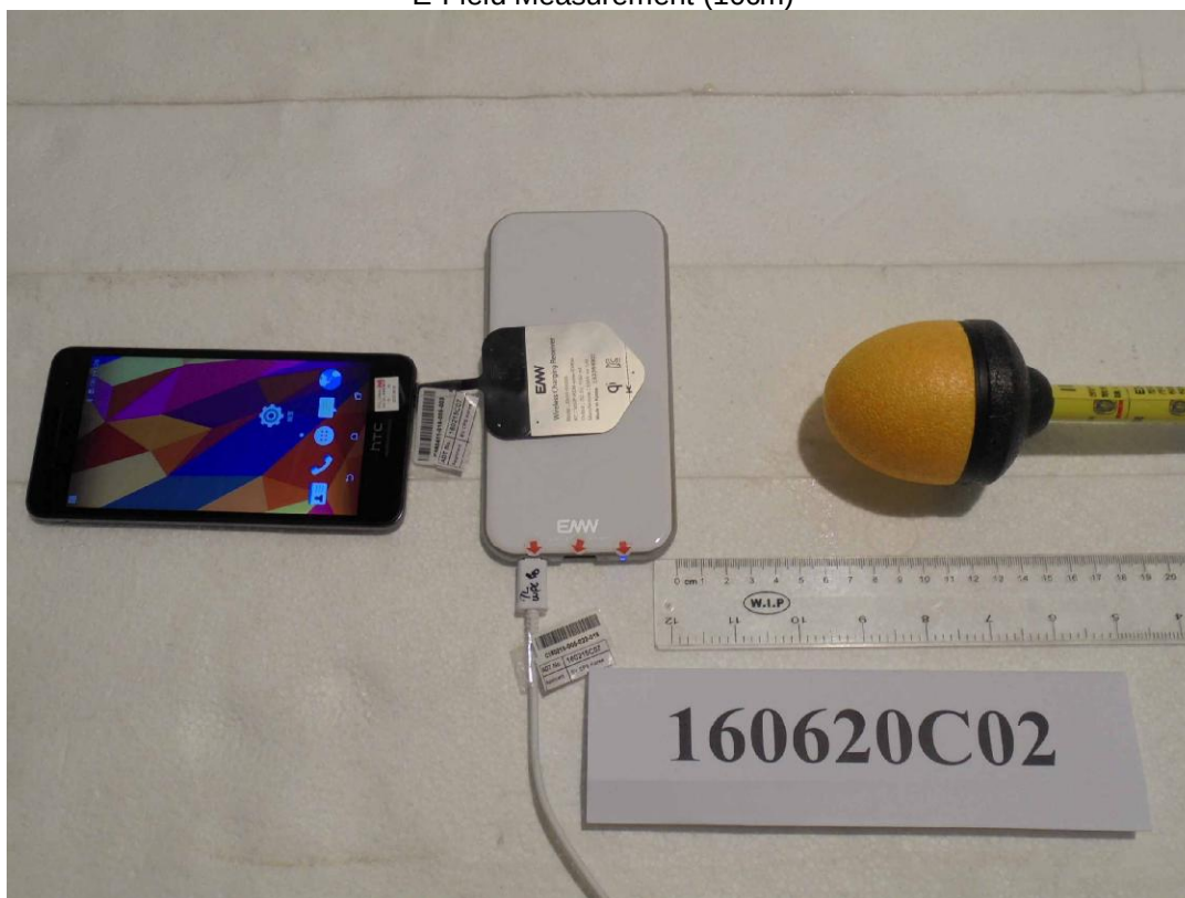
E-Field Measurement (10cm)
