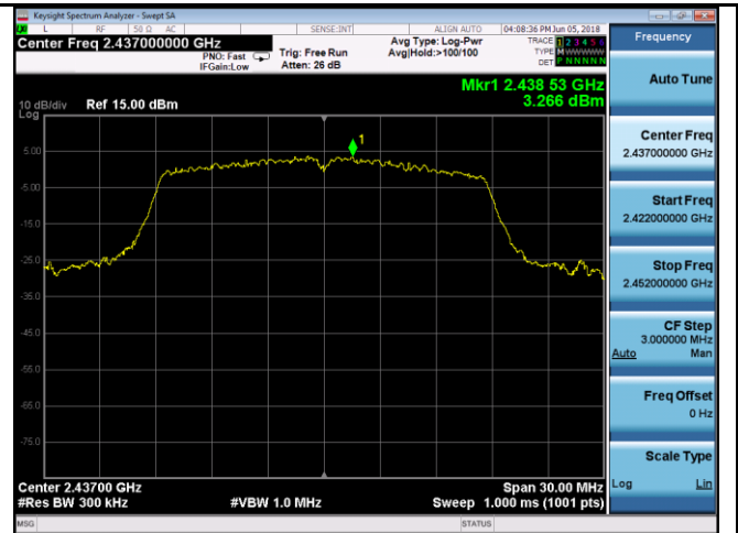
802.11n20 - PK Output power - Mid CH 2437
