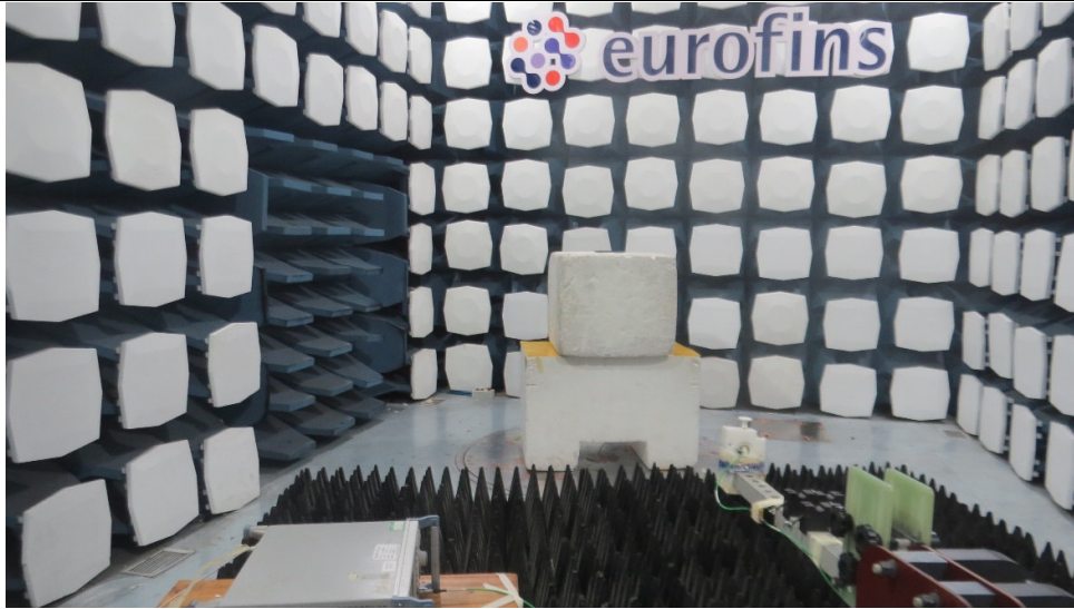
Picture 1 Radiated Emission Test Setup
