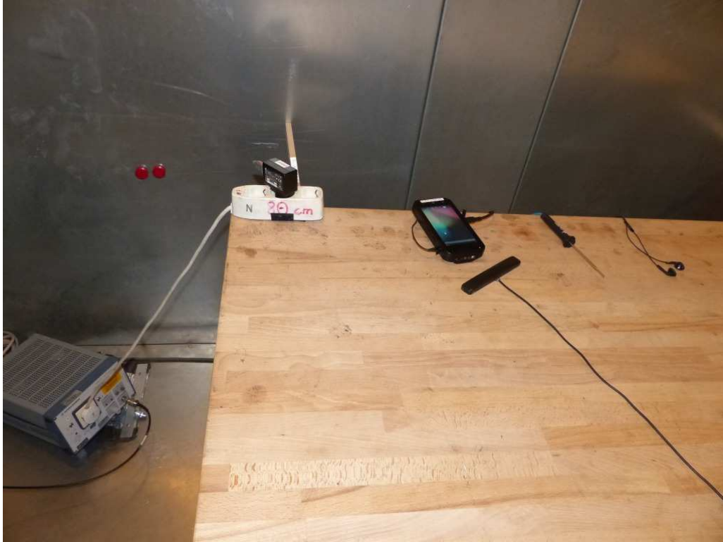
Photo 1: Test setup for conducted measurements (AC Port (power line), EUT Connected to the charger, intentional / unintentional radiator §15)
