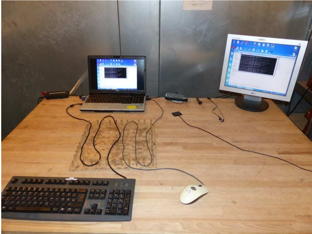
Photo 2: Test setup for conducted measurements (computer peripheral setup, EUT connected to the Laptop, unintentional radiator §15)
