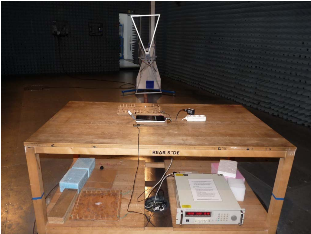
Photo 3: Test setup for radiated measurements (AC Port (power line), EUT supplied by AC/DC adapter, unintentional radiator §15)
