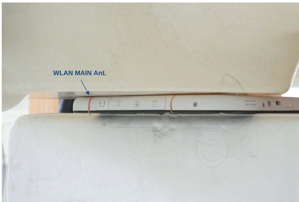
Fig. 26: Back side of Inari8-3GAN-1, 0 mm distance, WLAN MAIN antenna.
