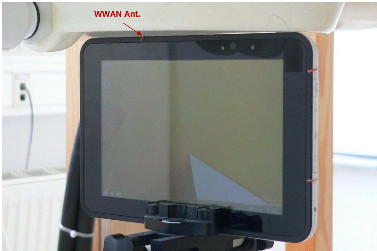
Fig. 25: Top edge of Inari8-3GAN-1, 0 mm distance, WWAN antenna, proximity sensor ON.
